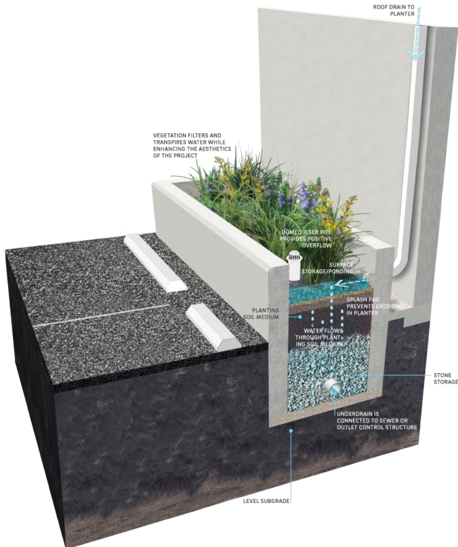
Figure 5.6. Illustration of bioretention with stormwater flow 191
