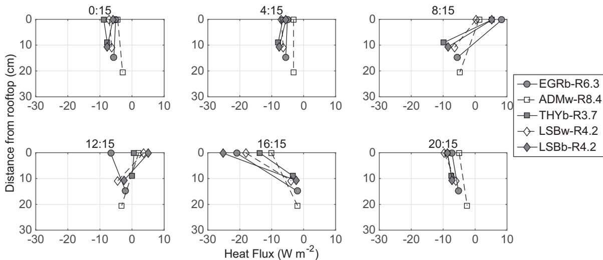
Fig. 6. Averaged heat flux profiles over different roof structures for January 2013.
