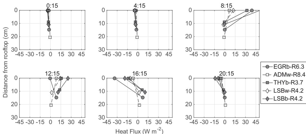
Fig. 4. Averaged heat flux profiles over different roof structures for August 2012; times in EDT (note that black roof markers are filled in gray and white roof markers are unfilled/white).
