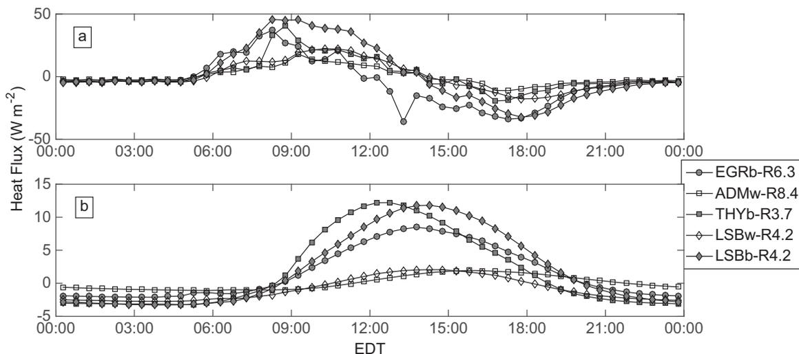
Fig. 7. Averaged diurnal variation of heat flux at the top (top panel) and bottom (bottom panel) of different roof structures for August 2012.
