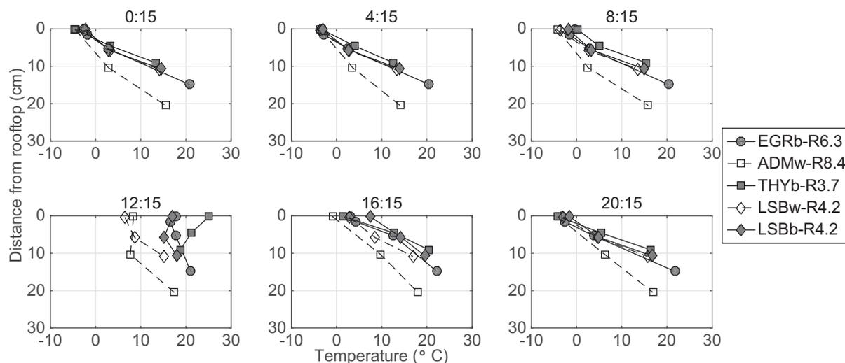
Fig. 5. Averaged temperature profiles over different roofs for January 2013.
