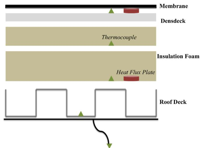
**Fig. 2.** An illustration of heat flux plate and thermocouple installation at PPPL—from the engineering building (the white spaces in between the layers are not air gaps, but are included in the figure for clarity of illustration).
