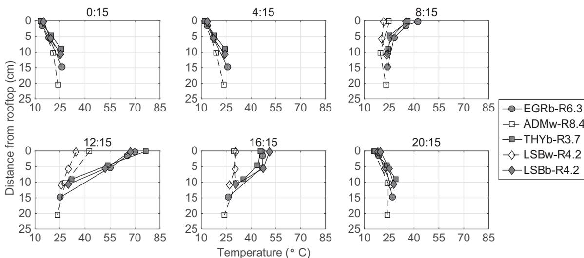
**Fig. 3.** Monthly-averaged temperature profiles at specific times over various roof structures for August 2012, time is EDT (note that black roof markers are filled in gray and white roof markers are unfilled/white).
