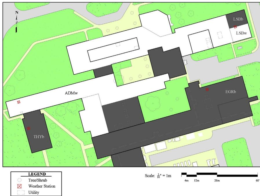
**Fig. 1.** Map illustrating the buildings and roof installation at PPPL test site. The sensors inside the roof layers were placed very close to installed automated weather stations, but at a sufficient distance to the south of the stations that ensured the roofs over the sensors were not shaded by the weather stations.
