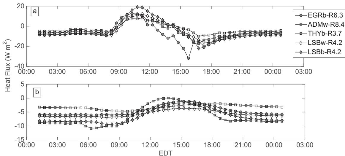
Fig. 8. Averaged diurnal variation of heat flux at top and bottom of different roof structures for January 2013.
