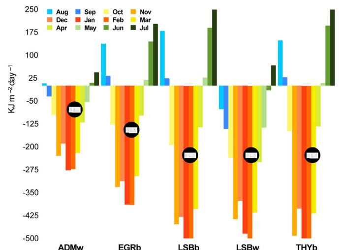
Fig. 9. Averaged daily heat flux in/out of roof structures from August 2012 to July 2013. A positive value indicates heat absorbed by the building while a negative flux indicates heat lost by the building.
