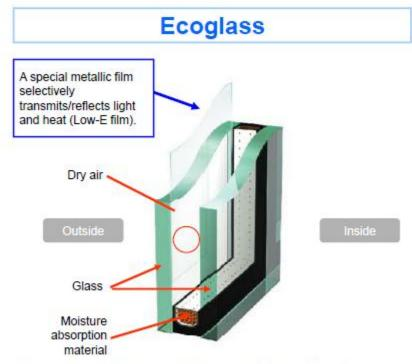
AGC achieved a greater heat insulating/shielding performance by placing a special metallic film (Low-E film) between the IG unit.
