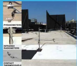
**Cool roofs last longer.** Temperature changes cause roofing material to expand and contract, causing basic roof wear and tear. Because black roofs reach higher temperatures than white roofs, they undergo higher levels of this temperature-induced stress and as a result, experience
