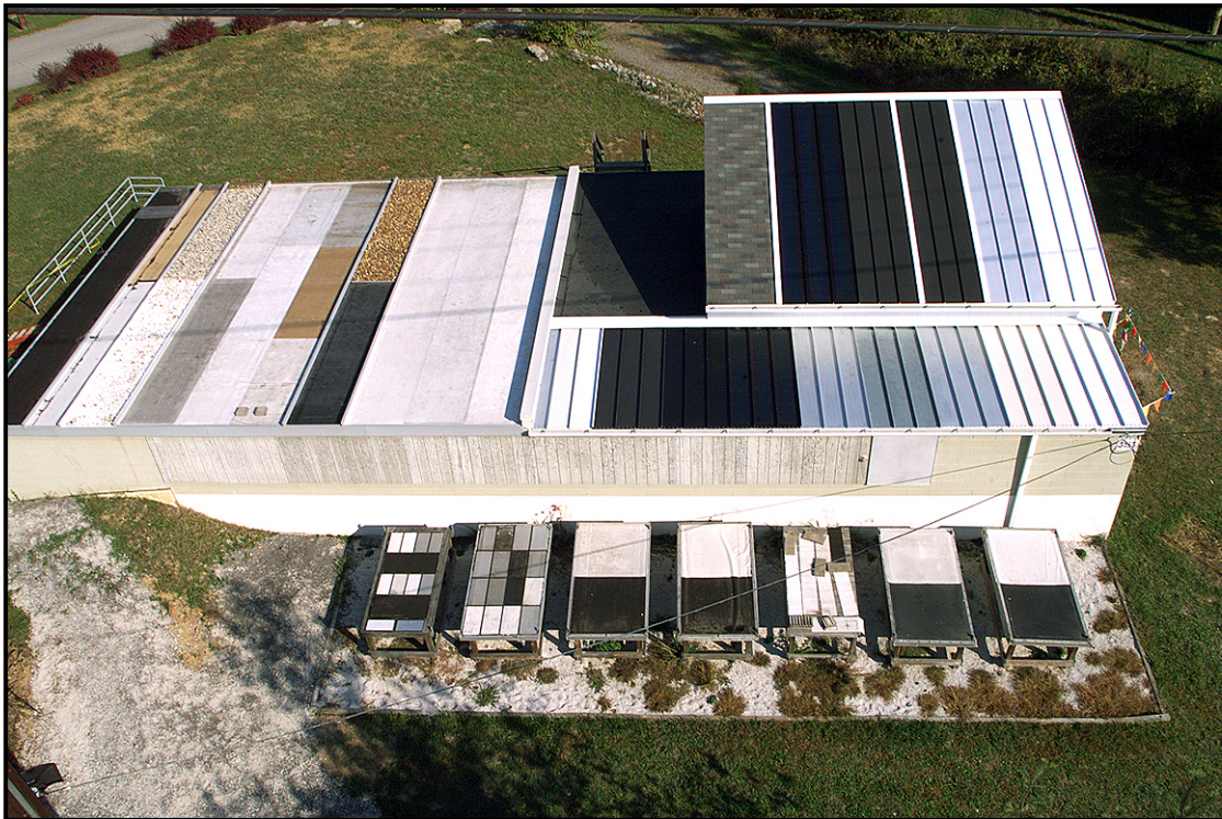
Fig. 1. The Envelope Systems Research Apparatus is used for testing roof manufacturer's best products.
