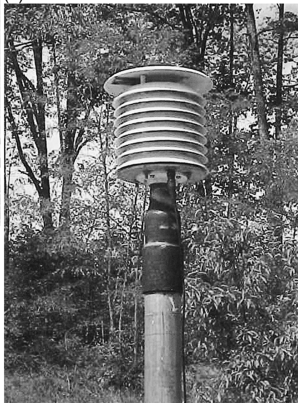
FIG. 3. (a) The HO-83 housing includes a small fan. (b) The painted wood CRS houses liquid-in-glass thermometers. (c) MMTS on a pole; this unspirated plastic shield is 24 cm tall. Photos courtesy of the NWS.
