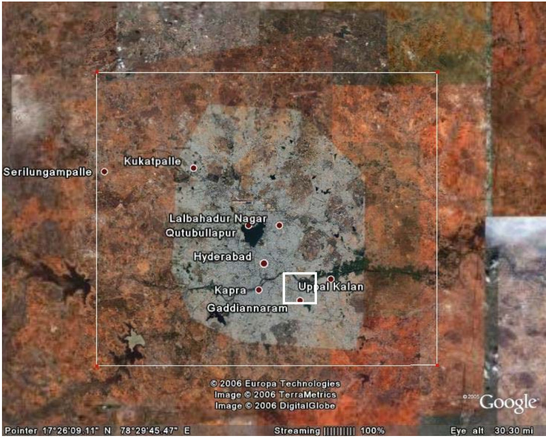
Figure 49. Sub-domain (dimensions: EW = 35 km, NS = 30 km) for 1-km LULC and surface characterization.
