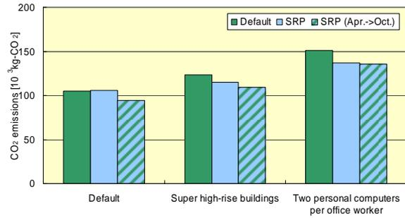
Fig. 12: Difference of CO<sub>2</sub> emissions by office automation (Office building)
