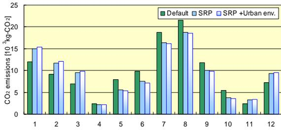
Fig. 9: Monthly CO<sub>2</sub> emissions from air-conditioning (Office building)
