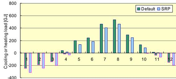
Fig. 4: Monthly cooling and heating load (Office building)
