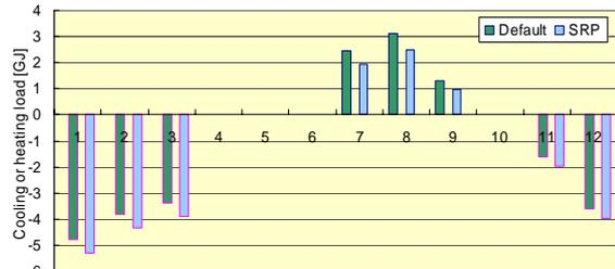
Fig. 5: Monthly cooling and heating load (House)
