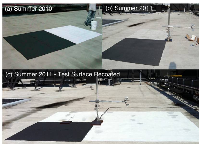
Figure 3. White roof conditions during the summers of 2010 and 2011 showing albedo loss effects over time. The original black membrane was first coated in summer 2009. (a) Surface conditions one year later after a fresh test patch was applied in summer 2010. (b) Surface conditions two years later just before sensor deployment began. (c) Surface conditions at the start of data collection after a second recoating.
